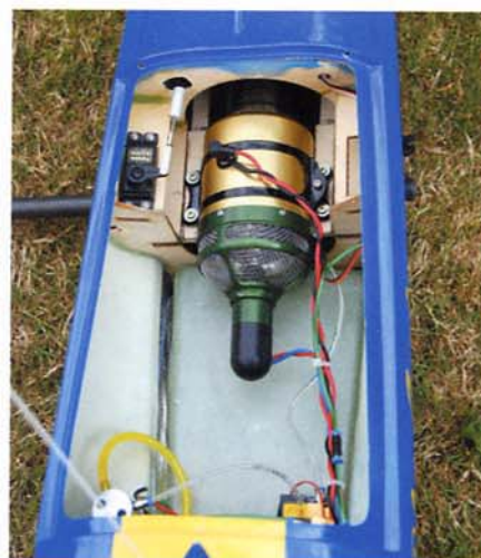
Engine installed with fuel tank in place secured with Velcro
