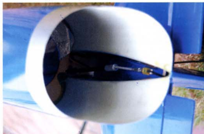
Torque rod for elevator operated by pushrod to servo by engine mount
