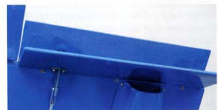
Split flaps should slow the model down well
