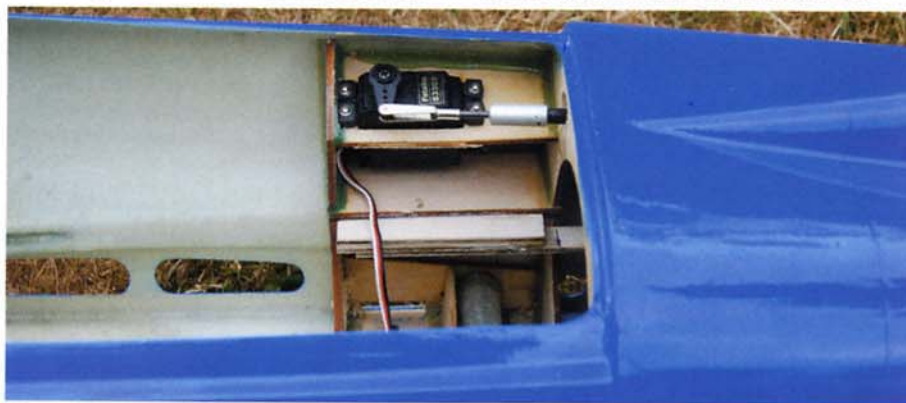
Elevator servo installed
