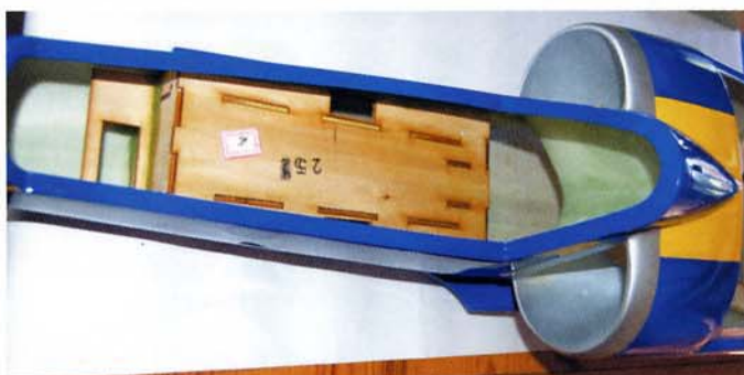
U/C ply box serves as mounts for steering, retract and brake servos
