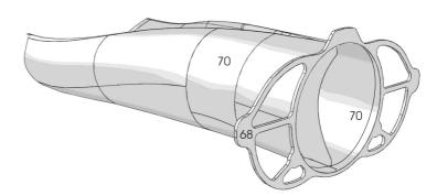
Tape the root facing ribs (14 + 15) to the front and rear fuselage sections (1 + 2) and fit the wing panels to check alignment. Note that the wing spars must be shortened by the thickness of the root facing ribs.
