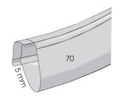
Glue the motor bulkhead (68) in the fuselage, flush with the end of the air ducts; reinforce the joints with additional rovings. The central connecting walls of the air ducts must now be glued together.
