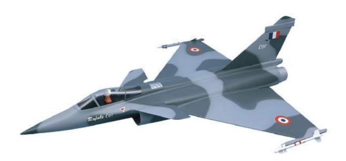
Specification Wingspan 940 mm Length 1340 mm Wing area 38 dm<sup>2</sup> Canard area  $3 dm^2$ 41 dm<sup>2</sup> Total surface area All-up weight 3200 g Total surface area loading 78 g/dm<sup>2</sup>
