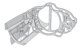
The wings can now be glued to the front fuselage section (1) and the root facing ribs (14 + 15). Apply two layers of 80 g glass cloth and resin to the joint area between the wing panels and the front fuselage section (1). Apply filler to the joint lines very carefully; these areas should not be sanded to avoid damaging the structural cloth.
